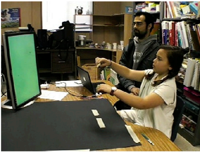
Figure 3. The MIT with hand-held IR emitters, which we found to be the most reliable means of hand tracking. A black matte surface on the desk helps reduce glare that can confuse the Wiimote's IR camera into seeing two IR sources. See http://tinyurl.com/edrl-mit2 for a 5 minute video clip showing the MIT in use.
